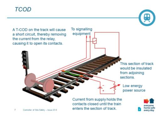
This diagram shows how the T-COD works by short-circuiting the Track Circuit it imitates the action of a train's wheels.
