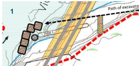
Work to be undertaken under low water conditions when there is no flood warning in place. Excavator containing bio hydraulic oils to slowly travel up the river and place the 1 tonne silt curtains. Once the temporary works are in place the remaining causeway material shall be removed.
