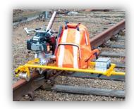
**13. Mobile Area Logistics Platform** (*Richard Merrills*) Rather than carrying tools and equipment down the track, this trolley fits onto the rails and can carry tools and equipment for you.
