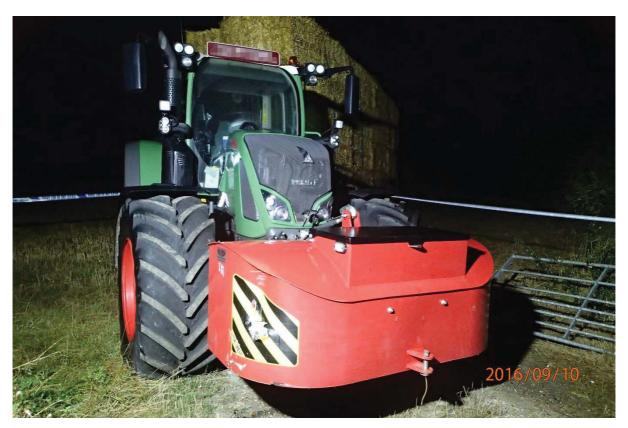
The tractor involved in the accident. The train hit the red counter-weight attached to the front
