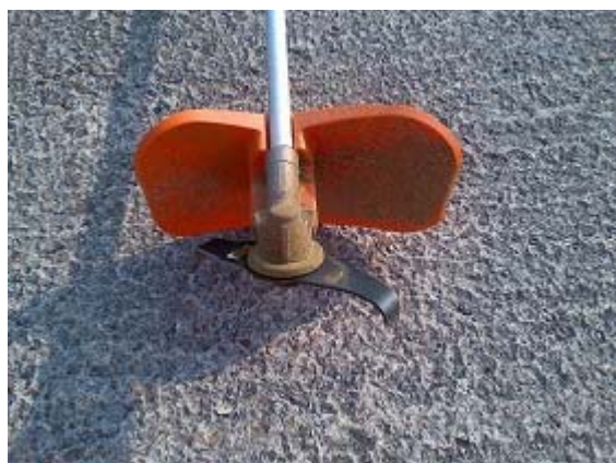
Figure 1 - Stihl brush cutter with shredder blade and correct protective guard fitted.
