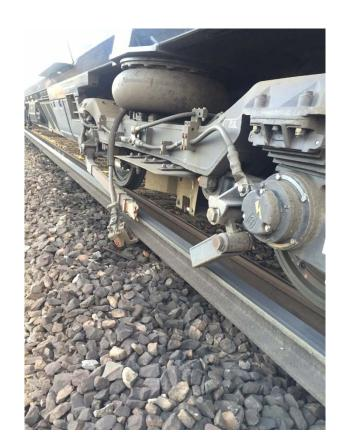
At 05.15 on 17<sup>th</sup> May following the hand back of a Thameslink Possession, the first passenger service travelling on the Up Charing Cross between Spa Road & London Bridge caught a traction cable with its conductor shoe.
