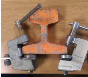
Approved clamp shown on left, non-compliant, ill-fitting clamp on right
