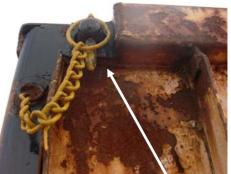
All pins must be in this position before the vehicle enters service
