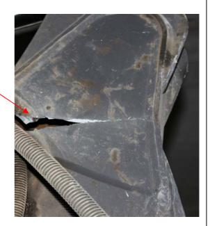
The pictures above show the failed dipper arm. The failure has been identified as a manufacturing fault with the dipper arm welding.
