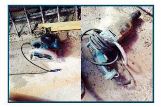
The tools were not only poorly maintained but were exposed on an open bridge in wet conditions.
