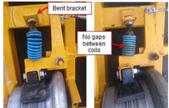
Link trolley failures
