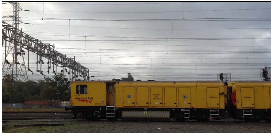
On track machine – rail grinder
