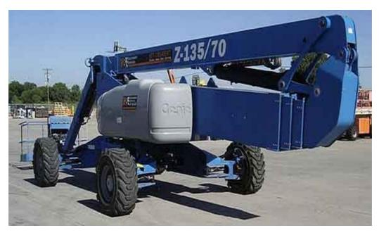
Genie have pro-actively updated the software for this machine. This updated software includes additional checks to the secondary lift calibration procedure without altering the physical calibration procedure or the operation of the machine. The updated software no longer tolerates a poor boom calibration and will lock the machine out if this condition is found.
