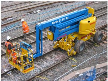
Action Required: Rexquote/Genie Z60/34 V3Accessrailers may now be used on Network Rail managed Infrastructure providing they have been modified by the manufacturer and have been tested with regard to interlocking and park brake performance.
