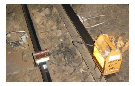
Product acceptance of the CRTLS (Box of Eggs) for testing the presence of voltage on conductor rails was withdrawn on 11<sup>th</sup> December 2012. To allow a phased introduction of
