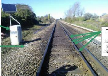
Four grease delivery blades on rail; the same arrangement is on the other side but obscured by shadow.
