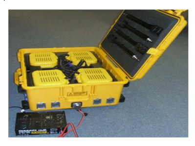
2. Equipment should be charged for the recommended time to achieve a full charge and then switched off. Equipment should not be left on charge for extended periods of time beyond that required to charge the battery to full.
