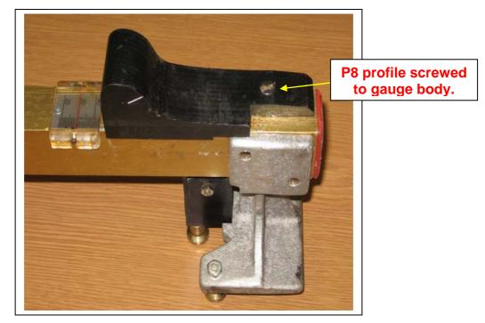
The screw attaching the P8 profile to the track gauge caused track circuit problems when the P8 profile was used
