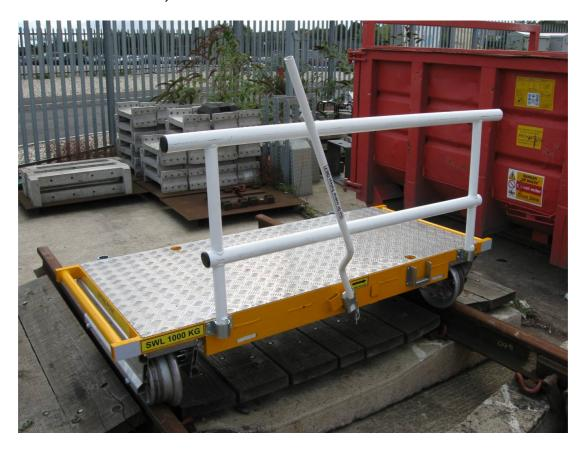
With reference to the Prohibition of these trolleys detailed in IGS Safety Bulletin 206, after investigation the derailment was found to be caused by the surface finish on the cast aluminium wheels. All 29 trolleys in service have had remedial work carried out to resolve this issue and all future trolleys supplied will have smooth wheels fitted when built.
