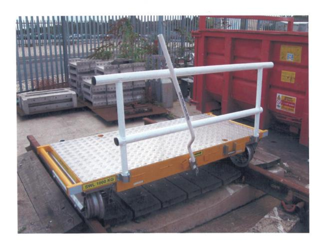
After a physical inspection and trial at Didcot it has been determined that under certain conditions these trolleys may have an increased risk of derailment and therefore pending further investigations any use of the Wolf Trakrat Trolley LT100P & LT1250A is prohibited until further notice.
