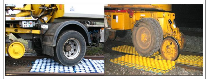
Standard **NR/L2/RVE/0007** was mandated in April 2007 and is intended to control and regularise the safe On/Off tracking of RRV's. It sets out 4 acceptable methods by which this may be done:
