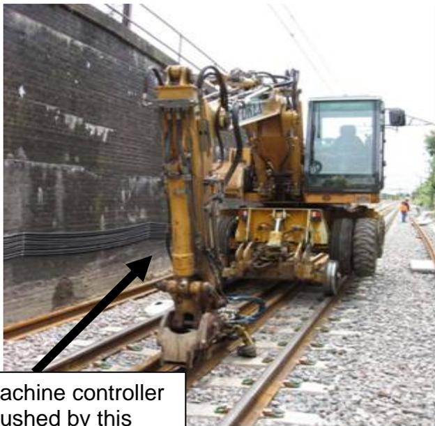
Machine controller crushed by this wheel set
