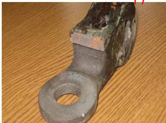
Figure 2. –Double Clevis shown in balance weight arrangement
