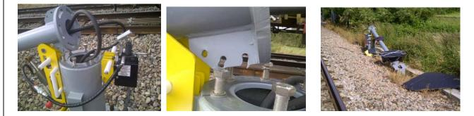
When the VMS Light Weight Signal is in its upright position it presents no risk, as there are no forces being applied at the jacking point.
