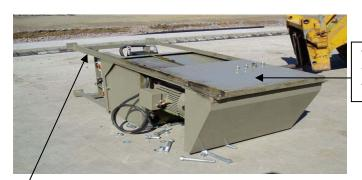
The majority of the load weight is positioned at the top of the equipment
