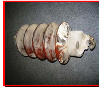
Figure 2: Flashover damage to top tube insulator
