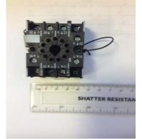
The strap added to the base should have been terminated between terminals 3 to 8 however it was fitted from 1 to 3 resulting in the 100 ohm resistor not being in the circuit as designed.
