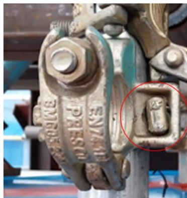
Fitting showing how the bolt head should have been seated in the clip body correctly to prevent fitting becoming loose and falling.
