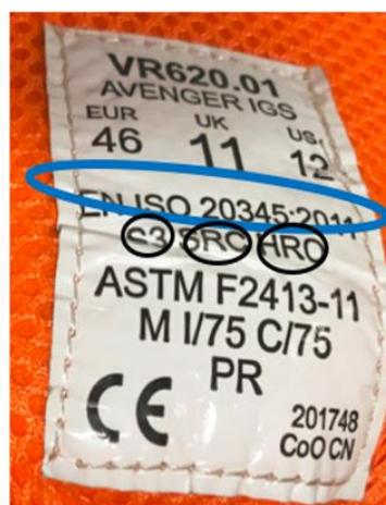
Footwear on site should conform to standard EN ISO 20345: 2011 Personal protective equipment – Safety Footwear. **S3 – midsole protection**
