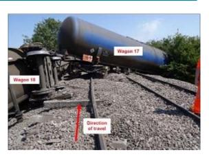
The separation of the train had caused the continuous brake pipe to part, applying the brakes to the train.
