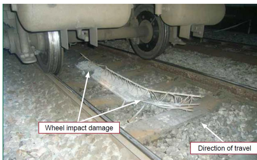
Plate 8: GE19 showing failed components having fallen from bridge over.
