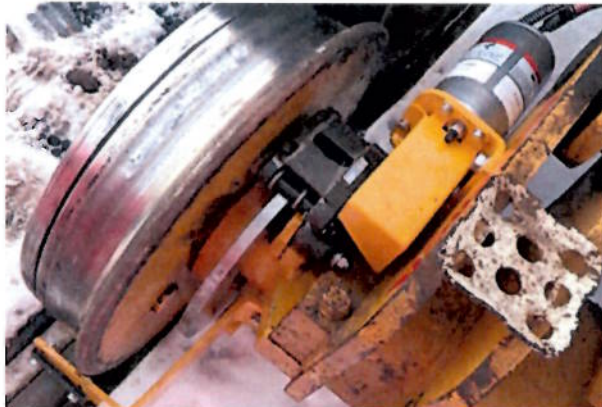
Picture 1 – Example of upgraded Type 9b RRV with Rail Wheel Brake system shown
