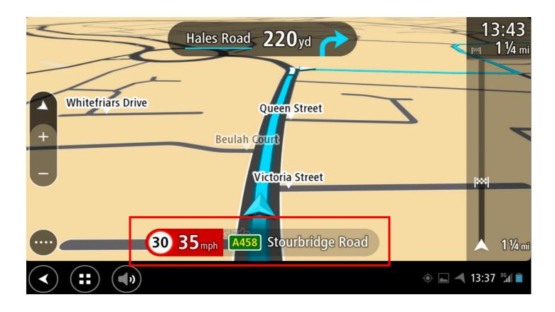
Within the navigation screen, drivers are made aware of the speed limit on that particular road on the bottom of the screen.
