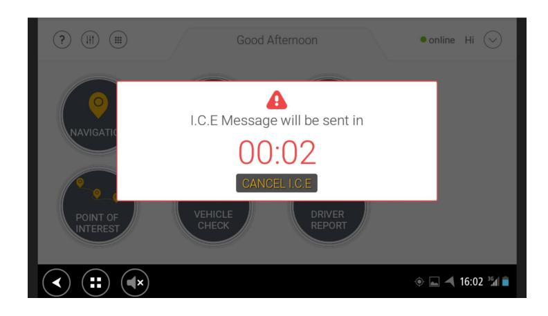
Drivers have access to an I.C.E alert to notify nominated contacts of an emergency. Once selected drivers have 5 seconds to cancel otherwise an alert is triggered.
