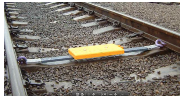
Eurobalise – used for various functions including APCO tilt activation (TASS), ETCS and Selective Door Opening (SDO) etc.
