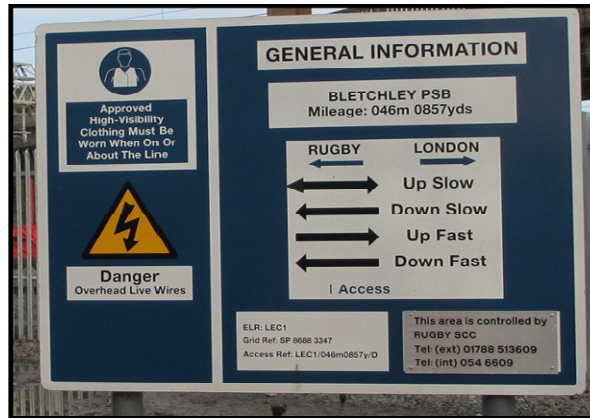
Typical example of Access information Signage in OLE areas
