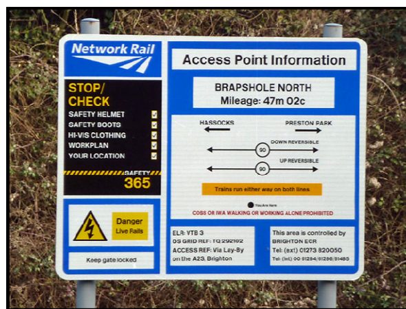
Typical example of Access information Signage in DC electrified areas
