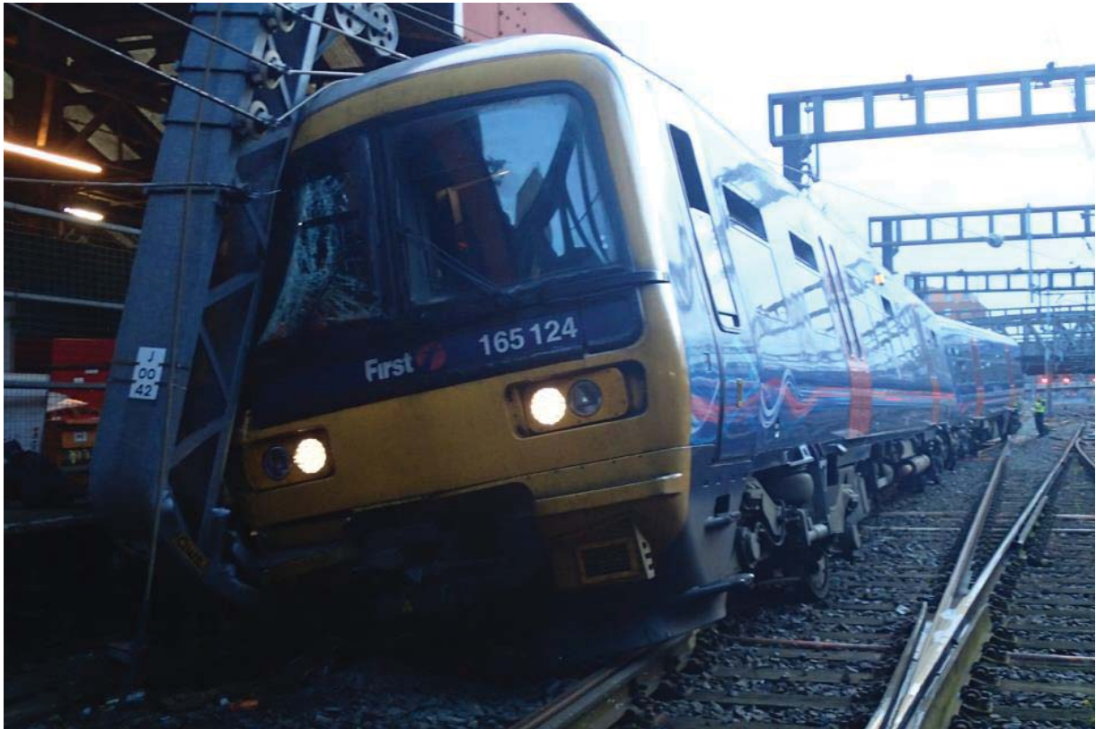
The front of the derailed train and the OLE mast, after the accident
