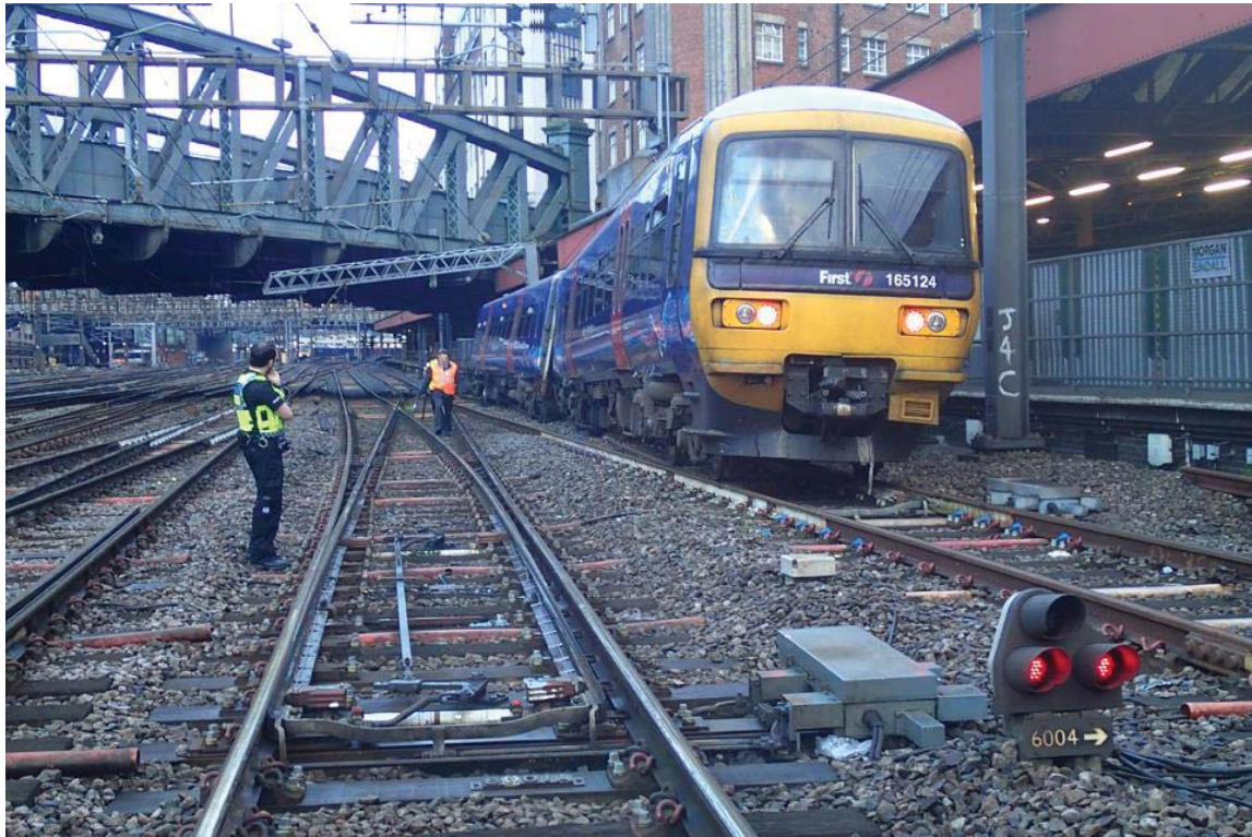
The train from the rear after the derailment. Signal SN6004 is at the bottom right
