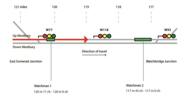
Simplified diagram showing relative positions of the speed restrictions (not to scale)
