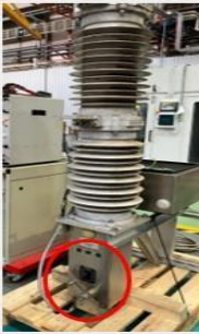
Rating plate in HV Pole, located at the magnetic actuator enclosure.
