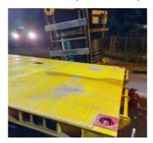
Position of the 'A' Frame after falling from the rail trailer
