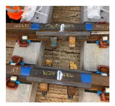
Rail clamps must be highlighted on SCPV wagon deck plans and positioned as such that they do not interfere with bearers, shroud plates and Cross beams (CrB). Only two rails may be fitted with rail clamps on the panel, with two clamps fitted per assembly.
