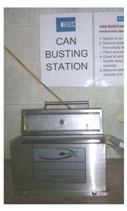
Constructed of stainless steel with a brass piercer, the handle is depressed to pierce the aerosol and the propellant is directed into the bottom chamber passing through carbon packs of varying sizes to extract as much as possible.
