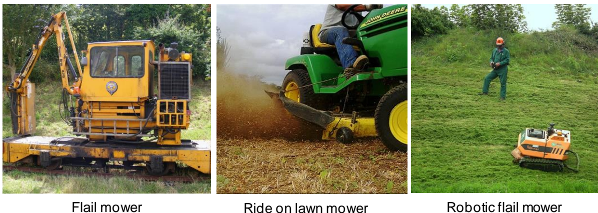
Figure 18 – Examples of grassland cutting machinery
