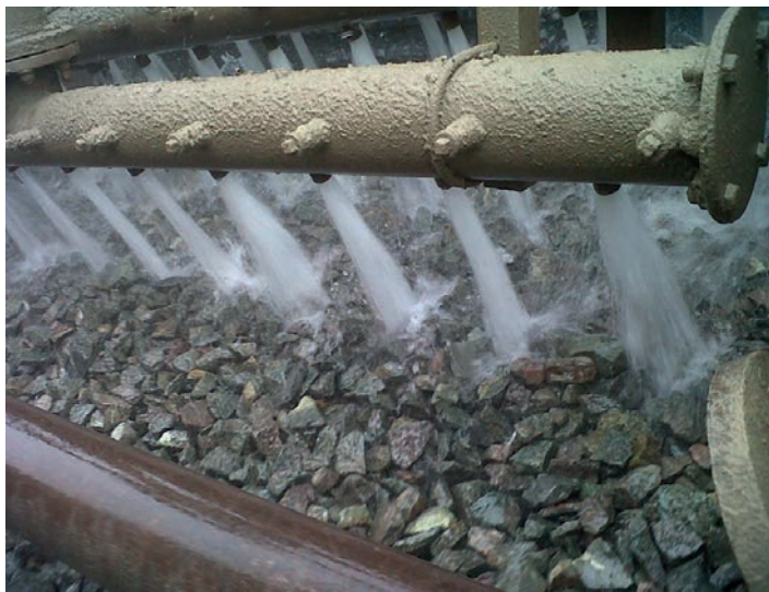
Washing ballast at the quarry
