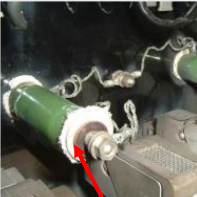
High Speed Circuit Breaker Resistors, Gasket
